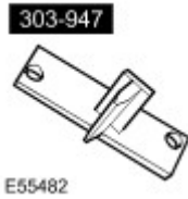
Flex plate locking tool 303-947 (LRT-12-145)
